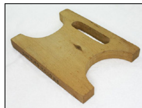
The spool to winding string around
